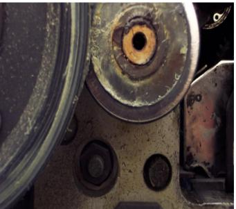
Over time, the roll pins holding the cam disc to the ink distributor roller shaft wear and become loose or even break. This allows the cam disc to rock back and forth which causes excess wear in the drive came and major damage to the shaft if not addressed in a timely manner.
